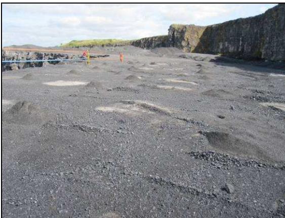
A bench that has been drilled ready to place explosives in the pattern of holes to blast the rock apart in a highly controlled operation.
